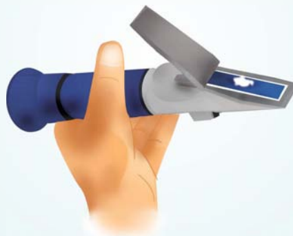
Clean the prism with distilled water and dry with a soft tissue to proceed with the next sample
